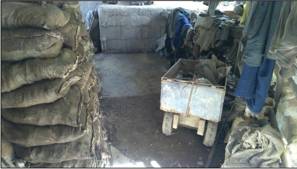
A mine car used for hauling ore, Ucab, Itogon.
